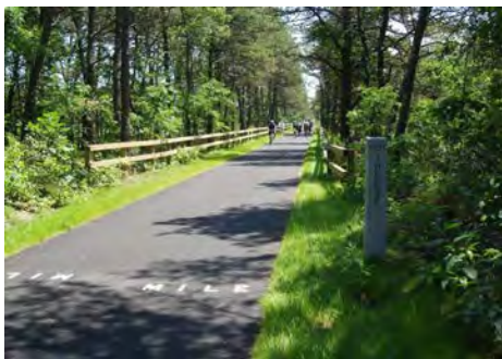
Minimize the maintained trail edge (2'-3' maximum width for lawn/low meadow buffer)
