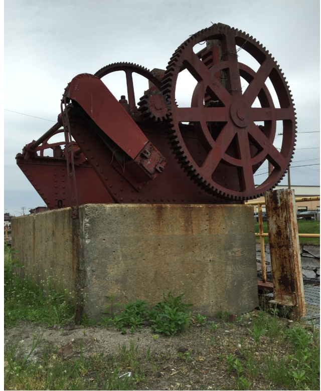
Figure III.6. Industrial relics: lock mechanisms on the South Canal.
