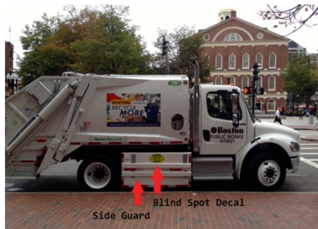
Figure A.13. Boston Public Works vehicle retrofitted with a side guards and convex mirror to minimize blind spots. These upgrades reduce risk of injuries and fatalities to bicycles in side collisions.
